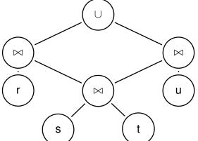
for each tuple in  $s\bowtie t$ , computation can be forked, joining it with r and u and contributing to the union in parallel
